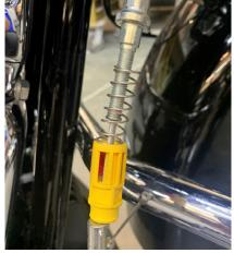
2. Remove the plastic adjustor from the upper cable with a a pair of side cutters. (The plastic adjustor is yellow on the 2021 models, and black on the 2022-2023 models). Cut the plastic from the bottom and from the top. Be careful not to cut the cable wire.
