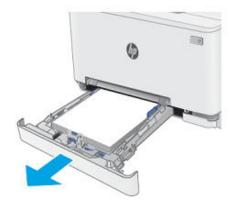
3. Push down on the single-sheet priority feed slot, and then pull out the feed slot tray.
