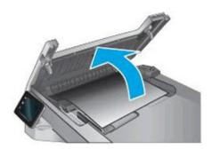
2. Remove any jammed paper visible in the input tray area. To avoid tearing any whole sheets of paper, pull the paper with both hands.
