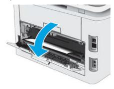
3. Use a flashlight to check for any paper or objects in the fuser area, and then remove any paper or objects you find. To avoid tearing any whole sheets of paper, pull the paper with both hands.
