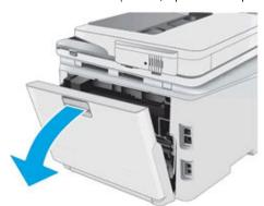
3. Use a flashlight to check for any paper or objects in the duplexer area, and then remove any paper or objects you find. To avoid tearing any whole sheets of paper, pull the paper with both hands.
