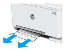
4. If no jammed paper is visible, or if jammed paper is deep enough in the Tray 2 area that it is difficult to remove, press down and remove the feed slot tray.
