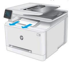
3. Use a flashlight to check for any paper or objects in the rear door area. To avoid tearing any whole sheets of paper, pull the paper with both hands.
