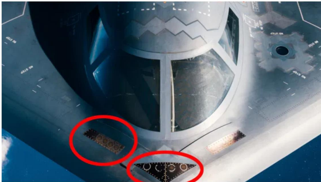
A close-up shot of the B-2 during AAR (Air to Air Refueling) shows the air data ports of the stealth bomber. (Original image: Staff Sgt. Jordan Castelan).
