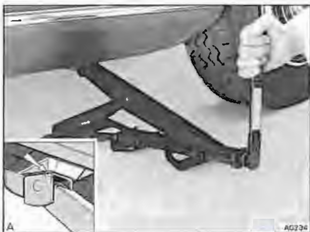
Fig. R2-3 Car jack correctly positioned
