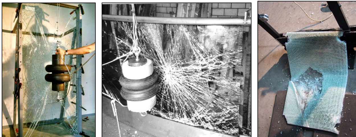
Figure 20 - Impact test EN 12600 (left), sufficient impact resistance of a curved laminated safety glazing balustrade with additional handrail at the top (center), failure example of a rather small, locally clamped, toughened glazing balustrade, punched-out as a whole (right) [2]
