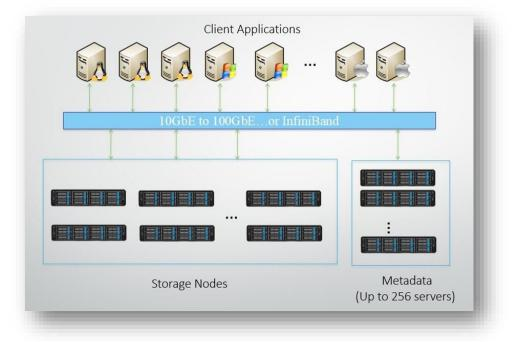
LeoFS was written to break away limitations from traditional storage solutions. It does not include concepts from legacy algorithms or other open source coding. The file system provides high performance for all workloads including big and small files, intensive reads and writes (random or sequential) and metadata heavy. Below is single cluster threshold.
