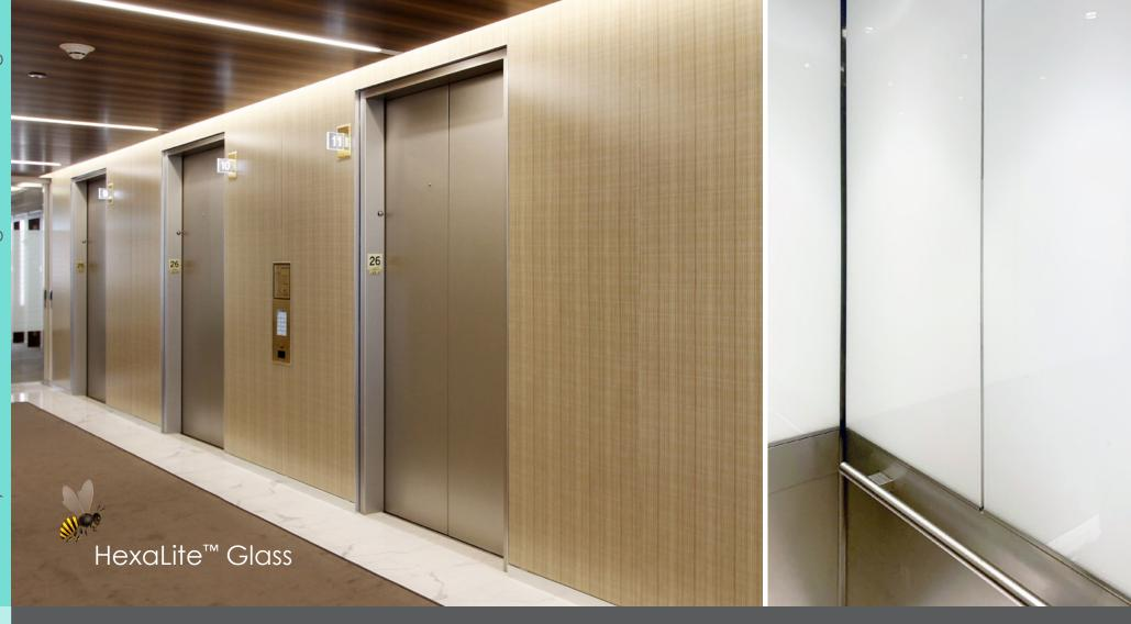
Honeycomb-reinforced glass by Bendheim is super-strong and ultra-lightweight. The laminated safety cladding material is ideal for elevator interiors, lobbies, feature walls, and designs requiring large glass panels and long spans.
