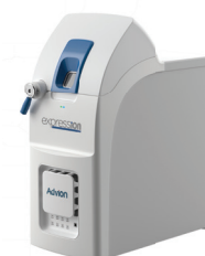
CMS Mass Spectrometer m/z range: up to 1200 (or 2000) single quadrupole mass spectrometer
