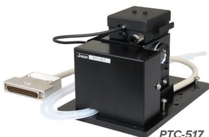
Three single-position Peltier thermostatted cell holders are available with a maximum light path length of 10 mm, to enable temperature control using the temperature control program. All feature a temperature setting range of -30 to 130°C with a measurement probe that can be placed inside or adjacent to cell and a magnetic stirrer to eliminate thermal gradients.
