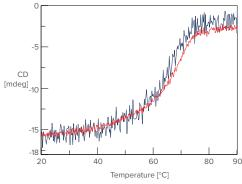
Tm measurement of Hemoglobin Wavelength: 222 nm Temp.: 20°C - 90°C
