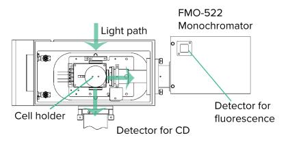
Above: Configuration for emission scanning with FMO-522
