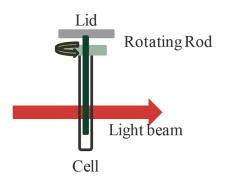
Figure 1. Schematic of the couette cell unit.
