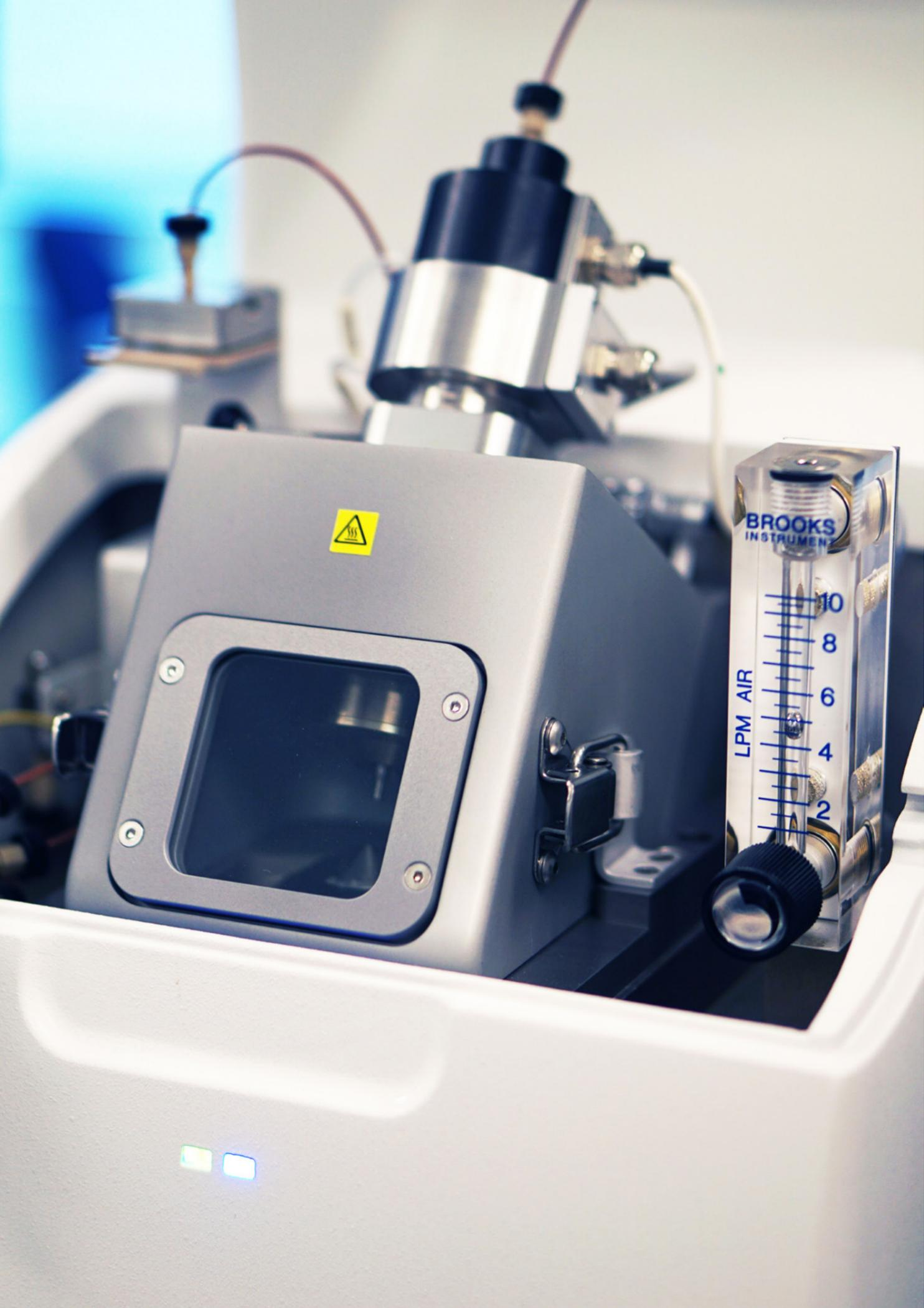
The LC-4000-MS mass spectrometry system has been developed to harness the power of a single quadrupole MS with an easy to use HPLC system.
