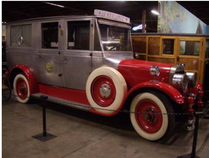
This ambulance was built by Jame C. Cunningham and Sons, Rochester, NY, and used in Bar Harbor, Maine, until the 1950s; it was also used as a hearse. Its body is made of hand-formed aluminum
