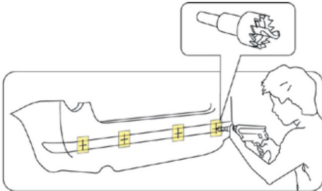
**Important.** Ensure that the sensors are mounted in the correct position at 90 degrees.
