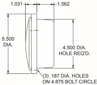
Back up lamps are available in incandescent and in both multi and single diode Multi-voltage. LED lamps are designed to operate for either 12 or 24 volt systems. Incandescent lamps use a 920139 lens with a 920460 socket and 1156 bulb. Multi-diode lamps use a 710037 LED clear lens assembly and the single diode lamp uses a 920139 lens with a 920691 single diode LED assembly.
