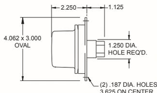
A back up lamp with a 1/4" N.P.T. threaded rear entry. Lamp features a Valox body with a 920112 deep clear lens with a press fit socket and 1156 bulb. Lamps are direct replacement to aluminum body version using a ground strap that utilizes the base of the lamp as a ground.
