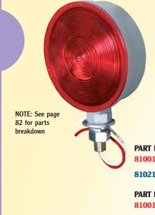
Pedestal mount aluminum body lamp is available in an incandescent and LED version. Incandescent bulb version features a 920134 red or 920135 amber lens. The single contact bulb version uses a 920015 single contact socket and 1156 bulb and the double contact lamp uses a 920013 double contact socket and 1157 bulb. The LED versions use a 710003 red or 710004 amber LED lens assembly.
