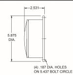
Back up lamps are available in incandescent and in both multi and single diode multi-voltage. LED lamps are designed to operate for either 12 or 24 volt systems. Incandescent lamps use a 920139 lens with a 920460 socket and 1156 bulb. Multi-diode lamps use a 710037 LED clear lens assembly and the single diode lamp uses a 920139 lens with a 920691 single diode LED assembly.
