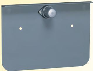
A grommet entry lamp 240002 comes attached to a gray powder coated 12 ga. steel license plate bracket 920062. Lamp features a silver 920055 lens and uses a 67 bulb.
