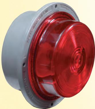
A tough valox body lamp available in an incandescent bulb or LED version. The incandescent bulb version features a 920141 red lens, a 920459 shock mount socket and an 1157 bulb. The LED version uses a 710025 Multi-voltage single diode lens assembly.
