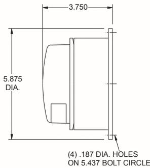
**PART NO. STOP/TURN TAIL OR CLEARANCE AND LICENSE DOUBLE CONTACT**
