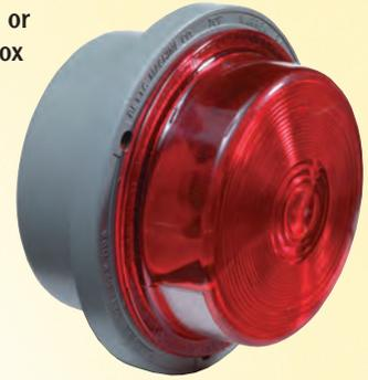
A compact size lamp available in both incandescent or LED. Lamp bodies are molded in a durable gray valox material. The incandescent bulb version features a 920141 red lens and uses a 920459 shock mount socket and 1157 bulb. The LED version is only available in valox and uses a 710025 Multi-voltage single LED lens assembly.
