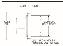
An incandescent lamp molded in durable gray valox. Features a 920113 red lens and a uses a 920104 shock mount socket and 67 bulb.
