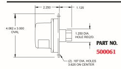
A self grounding valox body lamp that features a 920113 lens. Uses a 920127 socket and 67 bulb. Provided with a 1/4" N.P.T. rear entry. Surface mount.
