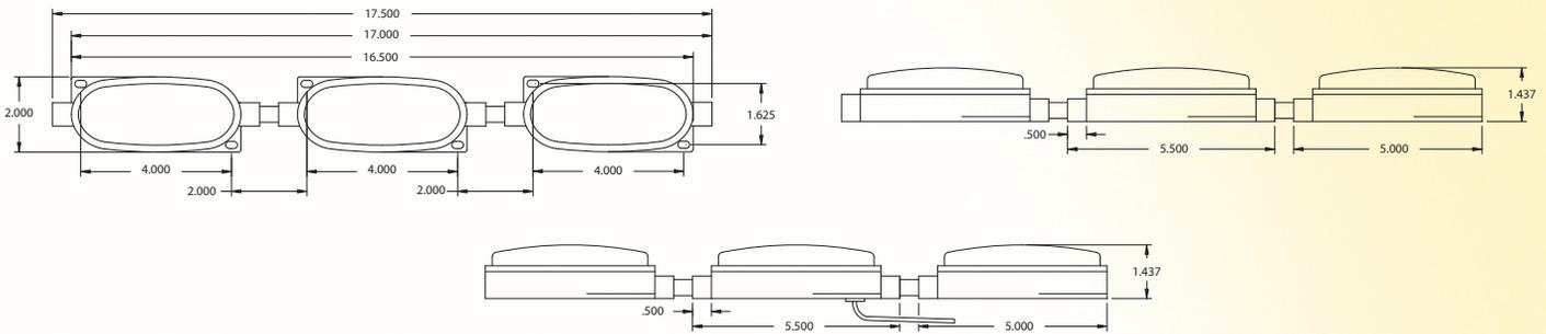
Features (3) REFLEX 920058 red or 920059 amber lenses and a tough valox body. Incandescent bulb version has a bulb replaceable shock mount socket and brass inserts with machine screws for a positive connection and uses (3) 168 bulbs. Surface mount.
