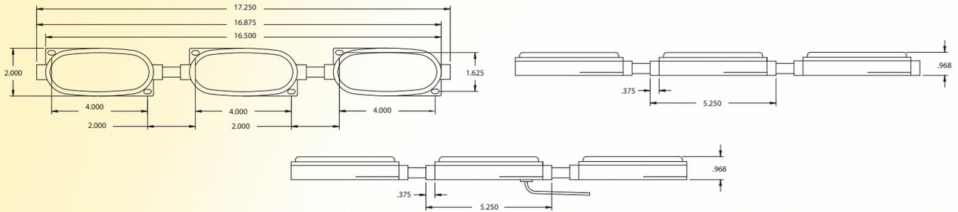
A low profile ID Bar lamp available in single contact incandescent bulb or LED version. The incandescent lamp features (3) 920049 red or 920050 amber lenses and uses (3) 67 bulbs.
