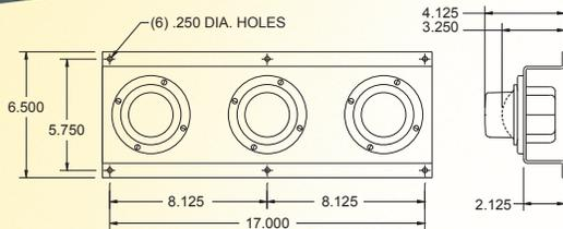
Lamps are available in an incandescent or LED style lamp and can be configured into either a shallow or deep lens option. Lights are mounted in a 920380 powder coated steel frame.
