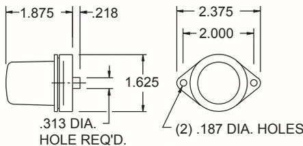
Features a 920053 red or 920054 amber deep lens. Lamps use a 67 bulb. Surface mount lamp with a .313 diameter wire entrance hole required.
