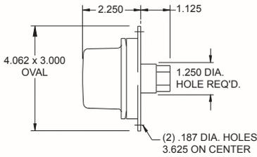
Available in either incandescent or LED, surface mount. Lamps have a 1/4" N.P.T. rear entry, surface mount lamp.
