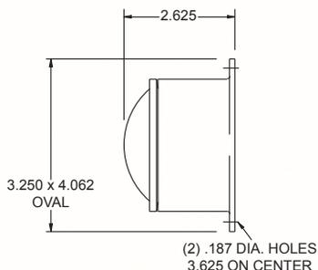
All 57 series lamps are molded from a durable valox material and must now be grounded internally by the use of an additional wire or by the use of a ground screw drilled thru the base of the lamp from the inside making ground contact using the socket or LED lens assembly ground wire and the metal mounting surface.
