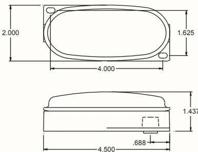
Incandescent lamp version features a REFLEX 920058 red or 920059 amber lens. The lamp features a bulb replaceable shock mount socket and brass inserts with machine screws for positive connections and uses a 168 single contact bulb.
