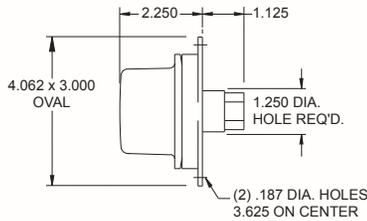
Special purpose double contact lamp deep lens incandescent or LED surface mount lamp. Lamps have a 1/4" N.P.T. rear entry.
