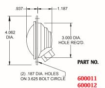
Incandescent version features a 920109 red or a 920110 amber shallow lens. Uses a single contact bulb socket 920125 and a 67 single contact bulb.
