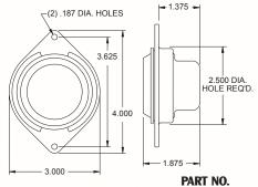
Incandescent bulb version features a 920228 red or a 920229 amber shallow lens and is available in a gray or black valox body. The 168 single contact bulb is mounted in a shock mount assembly for longer life. Provided with (1) or (2) 920413 watertight and vapor proof choke seals.
