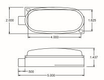
Incandescent bulb version features a REFLEX 920058 red or a 920059 amber lens. The lamp features a bulb replaceable shock mount socket and brass inserts with machine screws for positive connections and uses a 168 single contact bulb.
