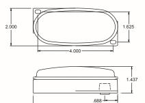
Incandescent lamp version features a REFLEX 920058 red or 920059 amber lens. The lamp features a bulb replaceable shock mount socket and brass inserts with machine screws for positive connections and uses a 168 single contact bulb.
