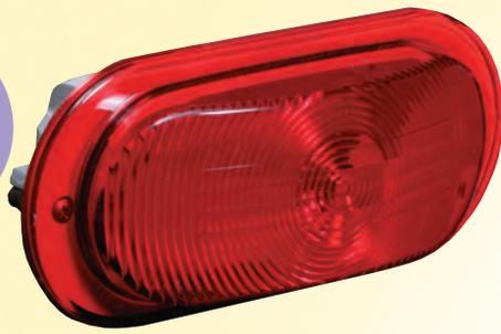
A tough nylon bodied lamp available in both an incandescent or Multi-voltage LED version. Both versions feature a 920454 red or a 920464 amber lens. The incandescent version uses a 920460 single contact socket and 1156 bulb or a 920459 double contact socket and 1157 bulb. The LED version features a 920685 red LED assembly for front or rear stop, turn, and tail. For amber, two assemblies are utilized - a 920686 LED assembly for a side turn and marker or a 920692 for rear turn only.
