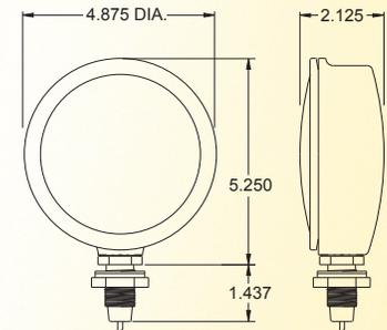
Requires a mounting hole large enough to accommodate a 3/4" diameter stud mount.
