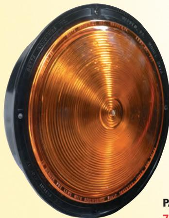
77 series lamps feature a valox body and are available in an incandescent or a red LED version. The incandescent bulb version features a 920152 red or a 920153 amber lens. The single contact lamp uses a 920460 socket and 1156 bulb and the double contact lamp uses a 920459 socket and 1157 bulb. The LED version uses a 920687 red LED assembly that can either be used as a single or double contact lamp.
