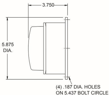
A surface mount lamp available in both incandescent and LED versions. The incandescent version features a 920144 red or a 920145 amber deep lens and uses a 920460 single contact socket and a 1156 bulb or a 920459 double contact socket and a 1157 bulb. The LED version uses a 710011 red or a 710012 amber LED lens assembly. Surface mount.
