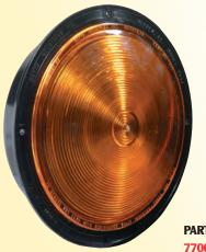
77 series lamps feature a valox body and are available in an incandescent or a red LED version. The incandescent bulb version features a 920152 red or a 920153 amber lens. The single contact lamp uses a 920460 socket and 1156 bulb and the double contact lamp uses a 920459 socket and 1157 bulb. The LED version uses a 920687 red LED assembly that can either be used as a single or double contact lamp.
