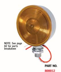
Pedestal mount aluminum body lamp available in a incandescent and LED version. Incandescent bulb version features a 920134 red or 920135 amber lens. The single contact bulb version uses a 920015 single contact socket and 1156 bulb and the double contact lamp uses a 920013 double contact socket and 1157 bulb. The LED versions use a 710003 red or 710004 amber LED lens assembly.
