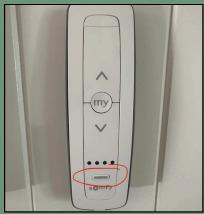
All studio blinds are electric with remote (located by front door). To change which blind is being controlled simply press the button circled in picture above and press up or down arrow.
