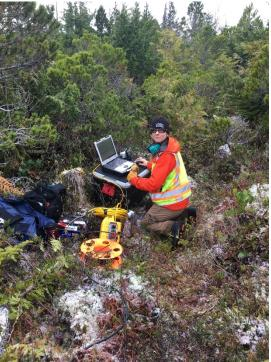
Ground-penetrating-radar surveys to measure ice (and snow) thickness on the North Slope of Alaska
