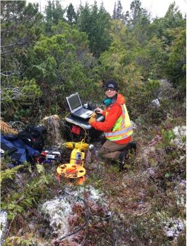
Seismic refraction surveys to measure depth to bedrock on Annette Island, Alaska
