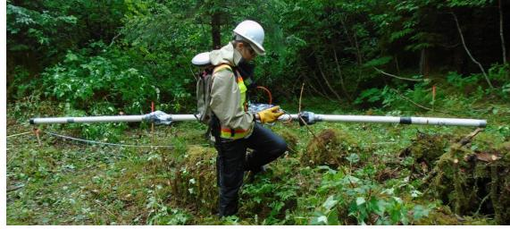
Using ground-penetrating radar (GPR) to find a buried ship
