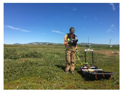
Seismic refraction surveys to measure depth to bedrock on Annette Island, Alaska
