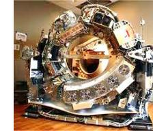
An existing design of a CT stationary gantry needed to have its natural frequency doubled to accommodate an operational speed increase.
