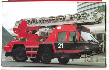
The Super Gyro Ladder is equipped with a conventional lifter and a rotating detachable basket at the top
