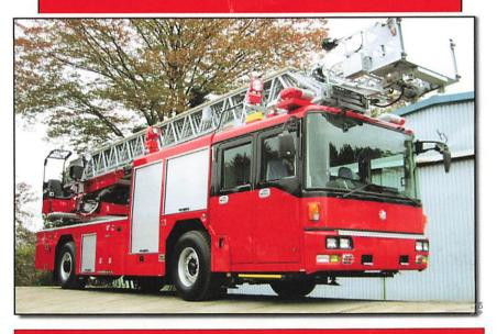
Sky Action Ladder is a vehicle with revolutionary characteristics, combining a snorkel ladder and a lifter
