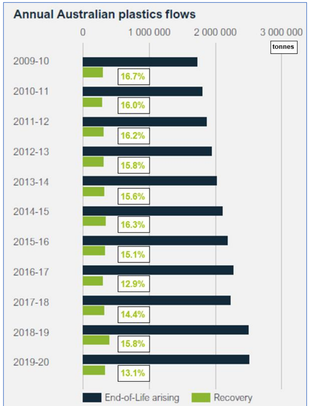
Figure B1.1 showing the tonnages of end-of-life plastic generated each year (in black) against the recycling rates (in green)
