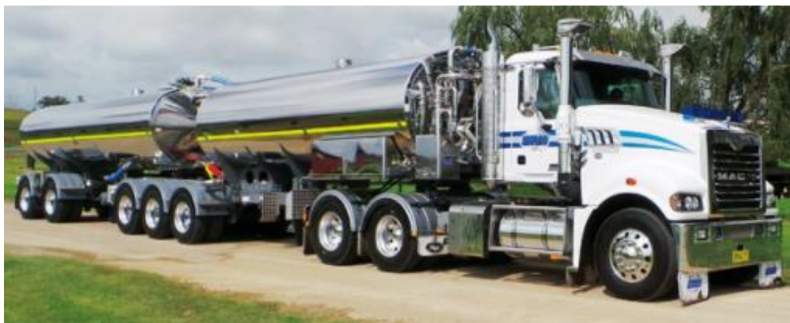
Figure C13.2 Typical B-Double 55 tonne capacity tanker truck to be used for Plasticrude transportation
