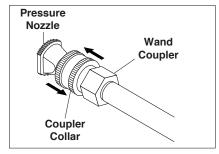
**STEP 4:** Release the coupler collar and push the nozzle until the collar clicks. Pull the nozzle to make sure it is seated properly.
