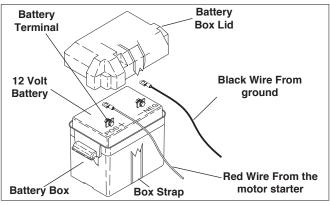
**STEP 8:** Place battery in battery box. Use a 12 V battery with a minimum capacity of 24AH.
