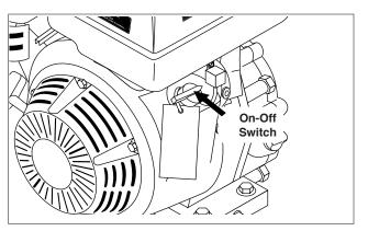
**STEP 8:** Turn the engine switch to "On" position.
