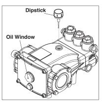
**STEP 2:** Remove shipping cap and install oil dipstick. Check pump oil level by using dipstick or observe oil level in oil window (if equipped). Use 40 wt. non detergent oil.
