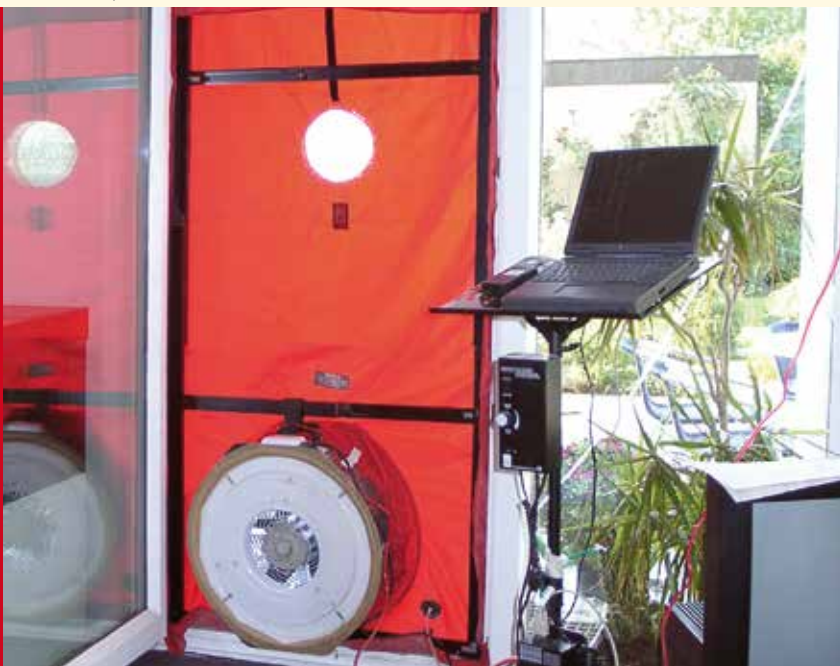
Fan for an air pressure test
