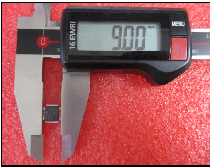
Dimension Measurement E=9.00mm(Pass)
