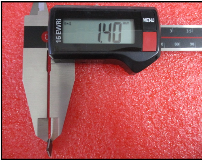
Dimension Measurement A2=1.40mm(Pass)
