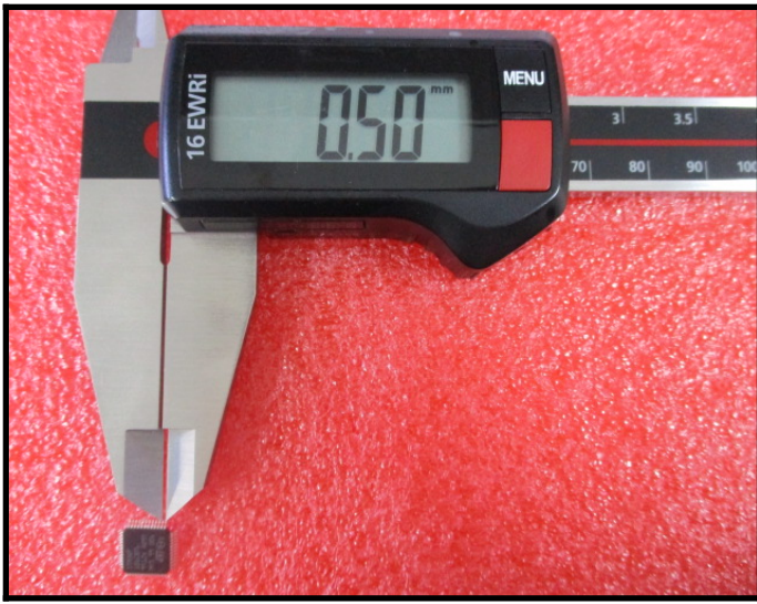
Dimension Measurement e=0.50mm(Pass)
