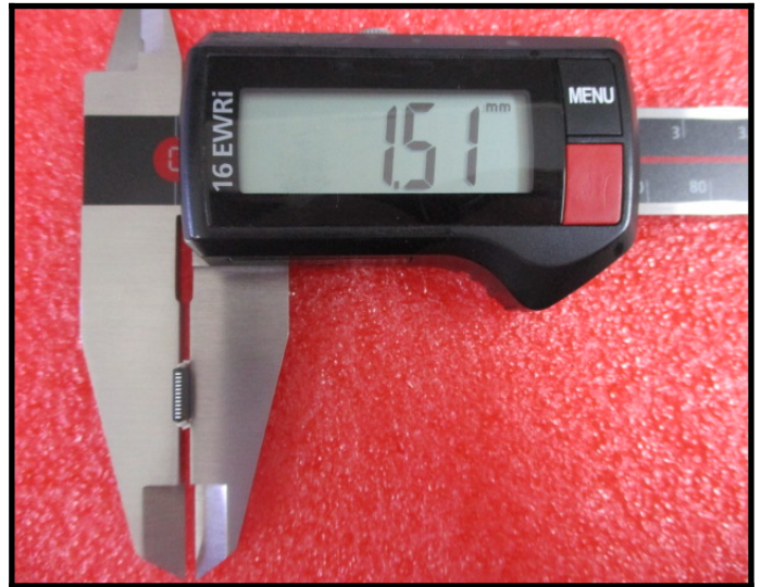
Dimension Measurement A=1.51mm(Pass)
