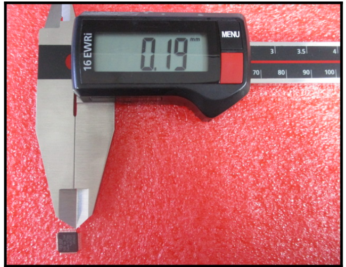
Dimension Measurement b=0.19mm(Pass)
