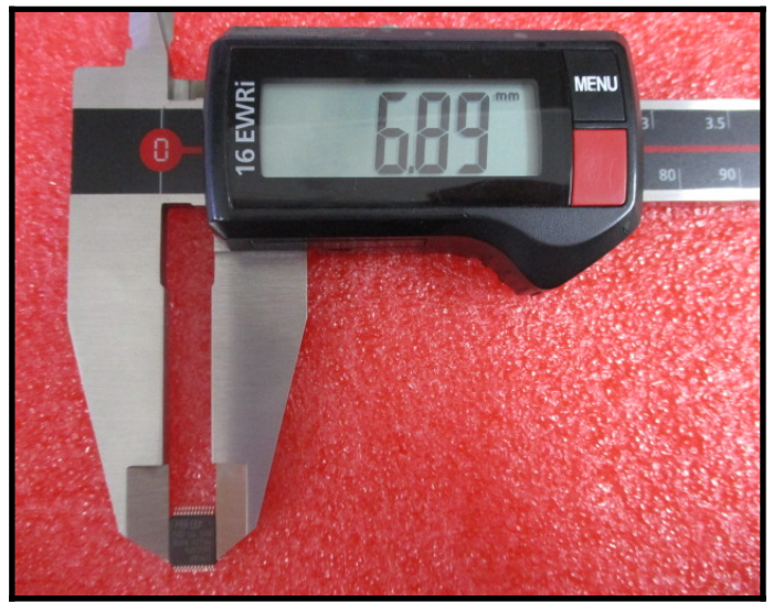
Dimension Measurement D1=6.89mm(Pass)
