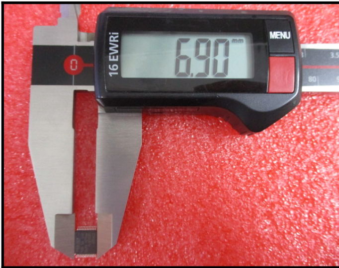
Dimension Measurement E1=6.90mm(Pass)
