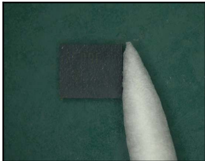
Marking (top-side) After chemical resurfacing test (Pass)
