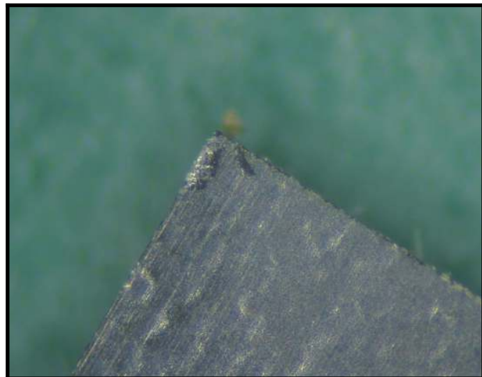
Marking (top-side) After mechanical resurfacing test (Pass)
