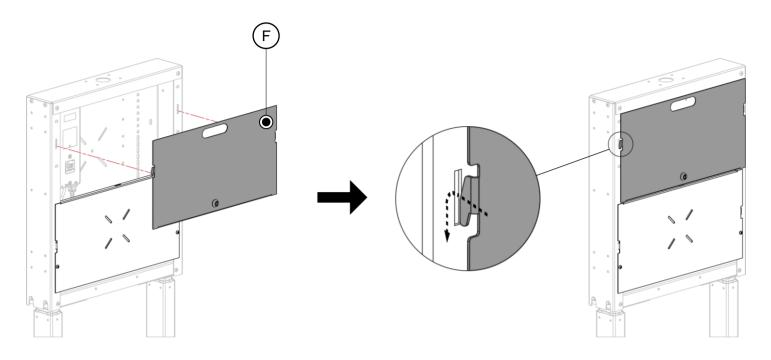
Insert one of the universal keys [D]. Lock the rear cover and remove the universal keys. Store the keys in a safe place.
