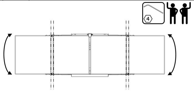
**8** Lock the position of each whiteboard by using 4x screw (F), use a power drill
