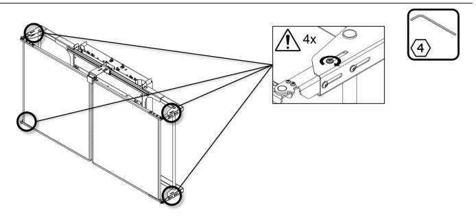
${f 3}$  Remove the screws at the side of all hinges, save the screws (G) (8x)
