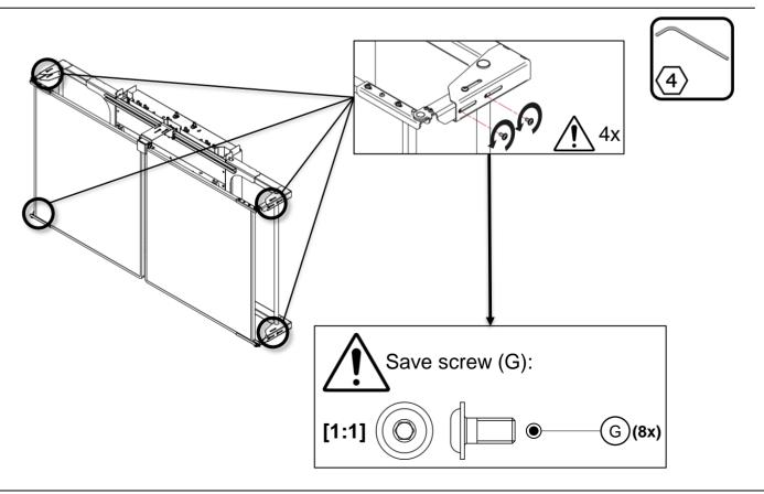
4 Mount 2x bracket (B) & 2x bracket (C) to the Winx-4b frame, use 8x screw (G)
