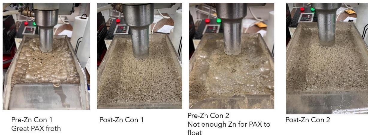
Figure 3.11 Flotation Test 1 – Zinc Stage Froth Photographs
