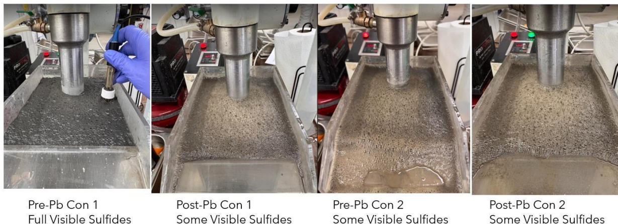
Figure 3.9 Flotation Test 1 – Lead Stage Froth Photographs
