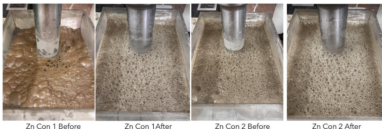
Figure 3.22 Flotation Test 2 – Zinc Stage Froth Photographs
