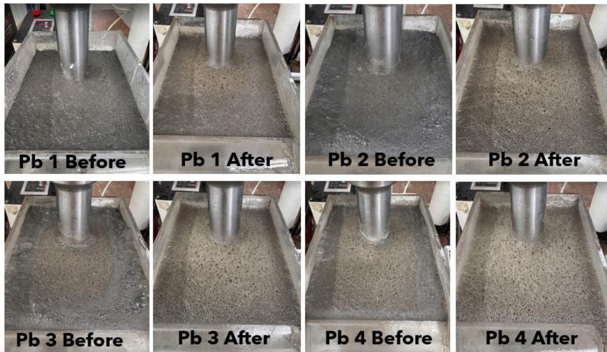
Figure 3.20 Flotation Test 2 – Lead Stage Froth Photographs
