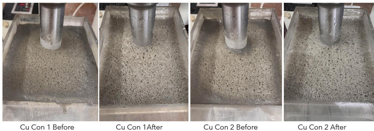
Figure 3.21 Flotation Test 2 – Copper Stage Froth Photographs
