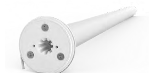
Automate Wire-Free Li-ion Zero Q1.1 5V, 1.1Nm, Ø25mm, 20-28RPM, 552mm long
