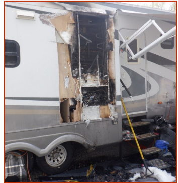
This 5th wheel fire was caused by a failure within the refrigerator.
