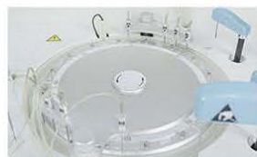
Reaction Tray 37±0.1°C, water bath
