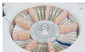
Reagent Tray 2~8°C cooling for 24 hours.
