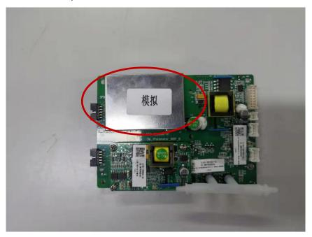
2. Unscrew the 2 screws on the SPO2 board to remove the board.
