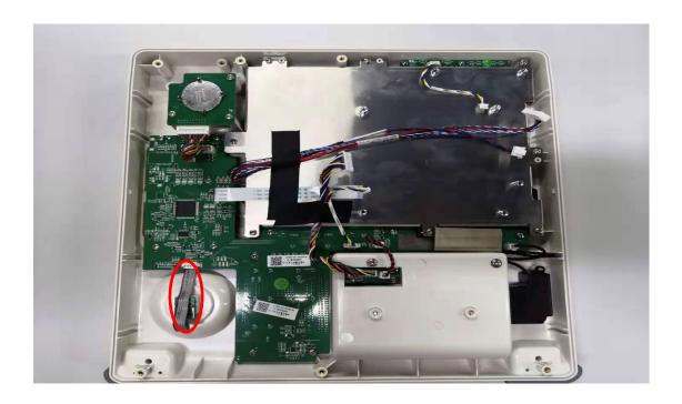
4. Remove the 12 PWA  $3.0 \times 5.0$ mm screws from keypad.
