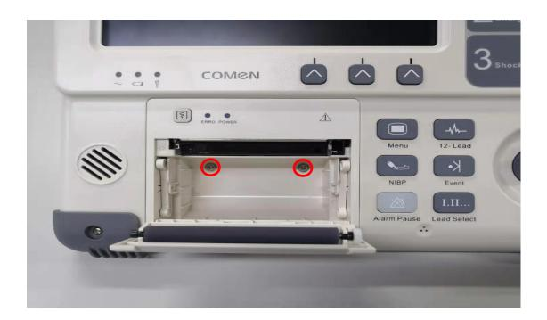
2. Remove the printer cable which connects to main board (socket: J32)
