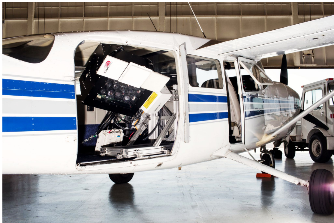
The surveillance camera array mounted on a Cessna 207
