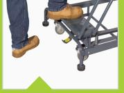
Apply 70 pounds of pressure to the steps & the ladder automatically drops the front feet to the ground securing the ladder to the floor for safe climbing.
