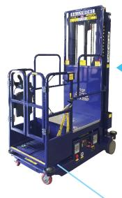
Power Stocker's optional sensing system creates a safety zone perimeter around the lift when in the raised position.
