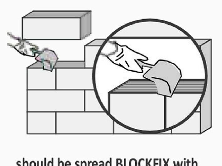
should be spread BLOCKFIX with 3-4 mm thickness
