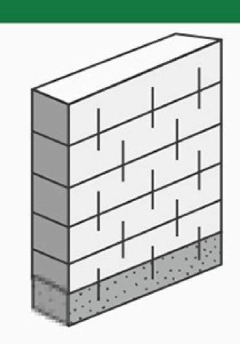
Do not disturb the wall after application of mortar for at least 24 hours.
