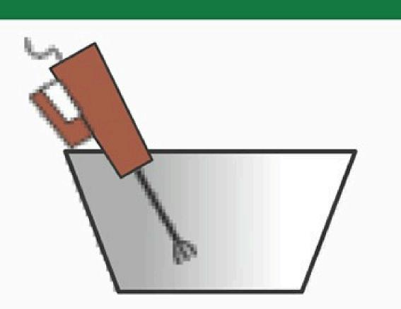
Mix first for 5-10 minutes by electrical mixer or hand tool mix homogeneously
