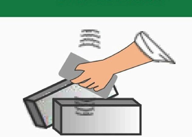
Before application clean the surface of blocks using suitable tools like brush so that any foreign materia is not held on the blocks.
