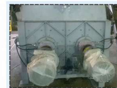
2 INDEPENDENT MOTORS WITH GEAR BOXES
