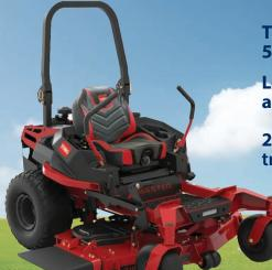
TURBO FORCE® Cutting Deck - 7-gauge steel, 5.5" deep deck.
