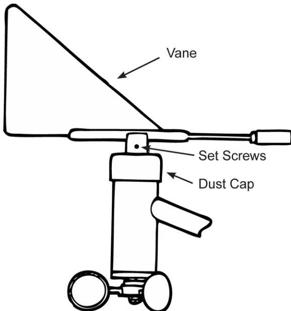
1. Once the sensor is plugged in, turn the cockpit instrument on. With the masthead sensor pointing in the same direction that it will be atop the mast, rotate the dust cap until the instrument reads "O", (needle is vertical). Hold the dust cap in that position.
