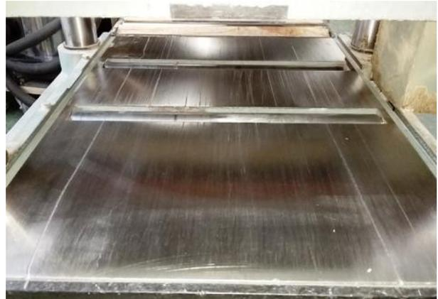
**ON A MORE SERIOUS MATTER:** Above right is a disappointing photo of the club's thicknesser which has received some abuse. It is obvious that something metallic has been embedded in wood that was put through the cutter resulting in deep gouges in the smooth surface of the plate. Please ensure that there are no **NAILS, SCREWS, STAPLES or STONES** in your wood before attempting to put it through the machine.
