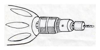
number of holes to be drilled the tape can wear, allowing the holes to become deeper. A piece of cork cut to the required length and twisted onto the drill-bit is a little more sturdy than the tape, easier to see and soft enough that it won't damage the timber being drilled. Worth a try.
