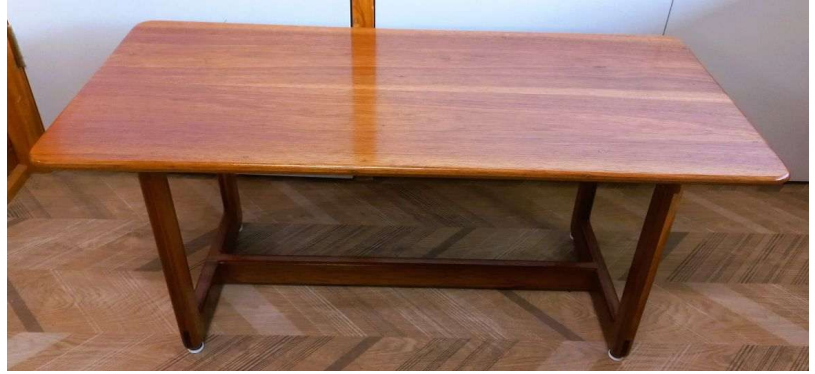
Lance Baker showed us the coffee table he made from recycled Tasmanian blackwood. The legs were laminated and joined with bridal joints, not mortise and tenon.
