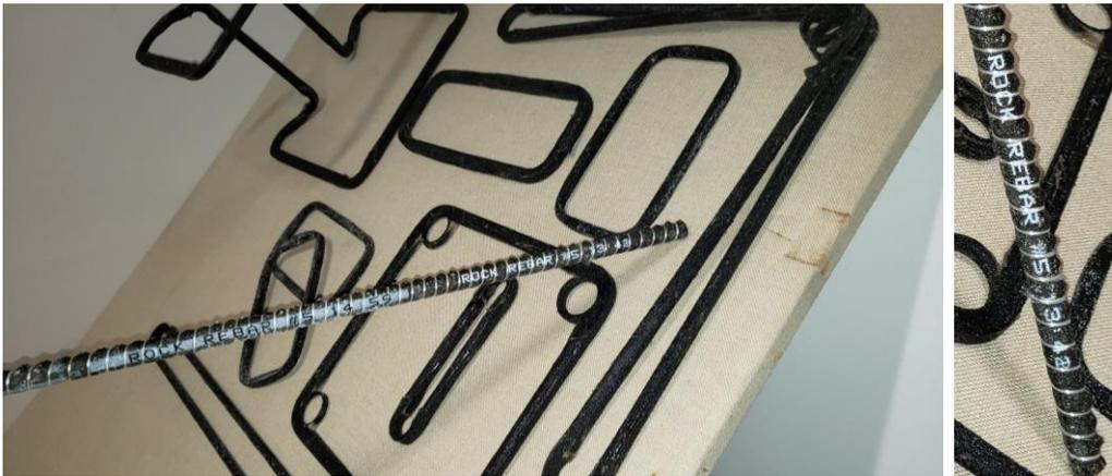
Figure 1 – BFRP made with Epx/ANHYD resin 'Rock Rebar' samples
