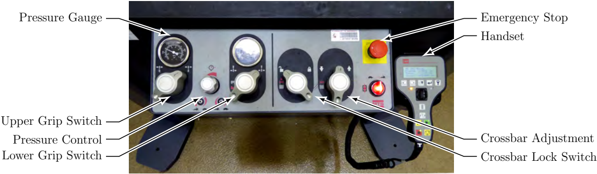
Figure 4.20: MTS control panel
