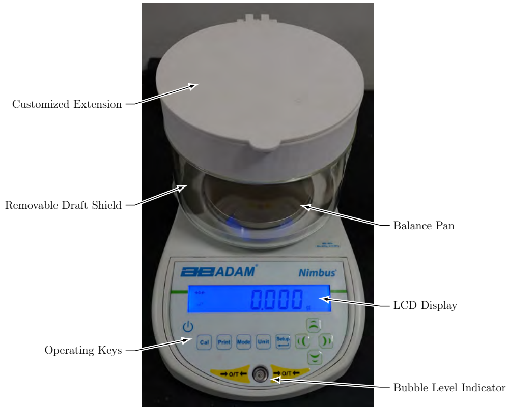
Figure 4.6: Precision scale, used to meet ASTM D 792 requirements
