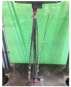
Figure 5.3 – Representative failure mode of tensile test
