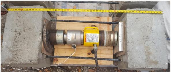
Figure 8.2 – Representative test setup for bend bar tests.
