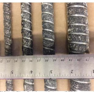
Figure 1 – RockRebar<sup>™</sup> Basalt Fiber-Reinforced Polymer (BFRP) composite reinforcing bar under evaluation, from left to right #3, #4, #5 and #8.
