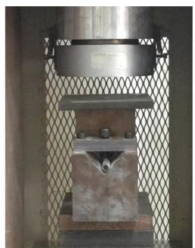
Figure 6.1 – Transvers shear strength test set-up
