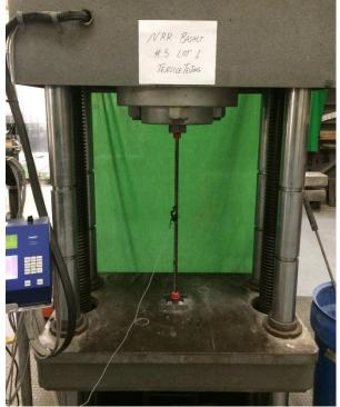
Figure 5.2 - Tensile test set-up
